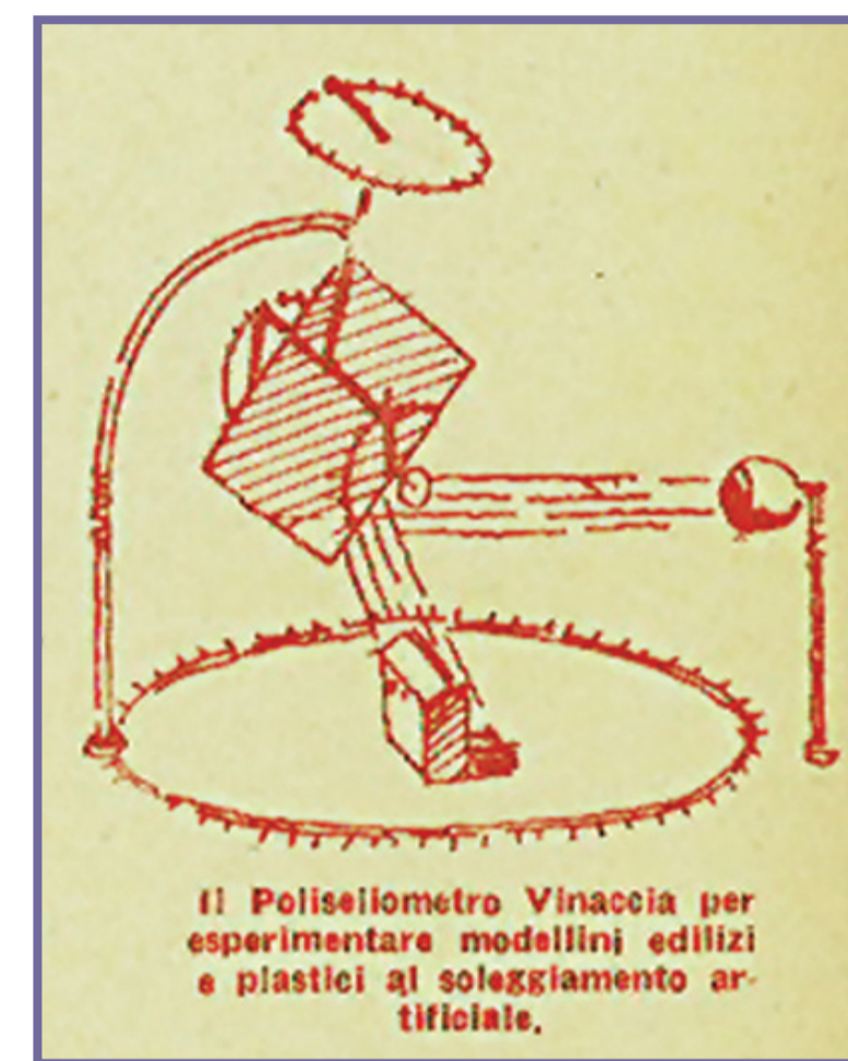
Fig. 5 - To orient buildings and streets he patented various devices as the poliesometro shown in this picture (1946).
