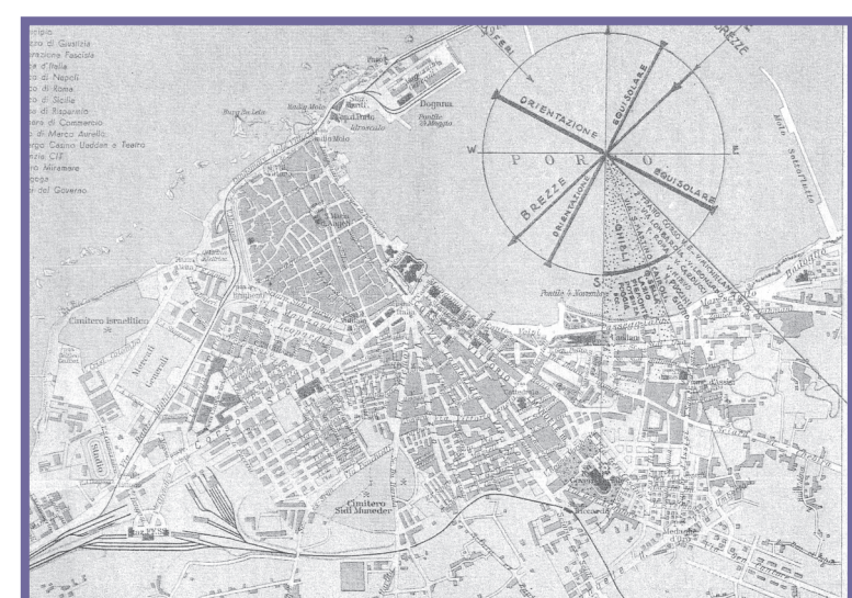
Fig. 4 - Vinaccia's study on solar orientation and wind directions for the urban plan of the city of Tripoli.
